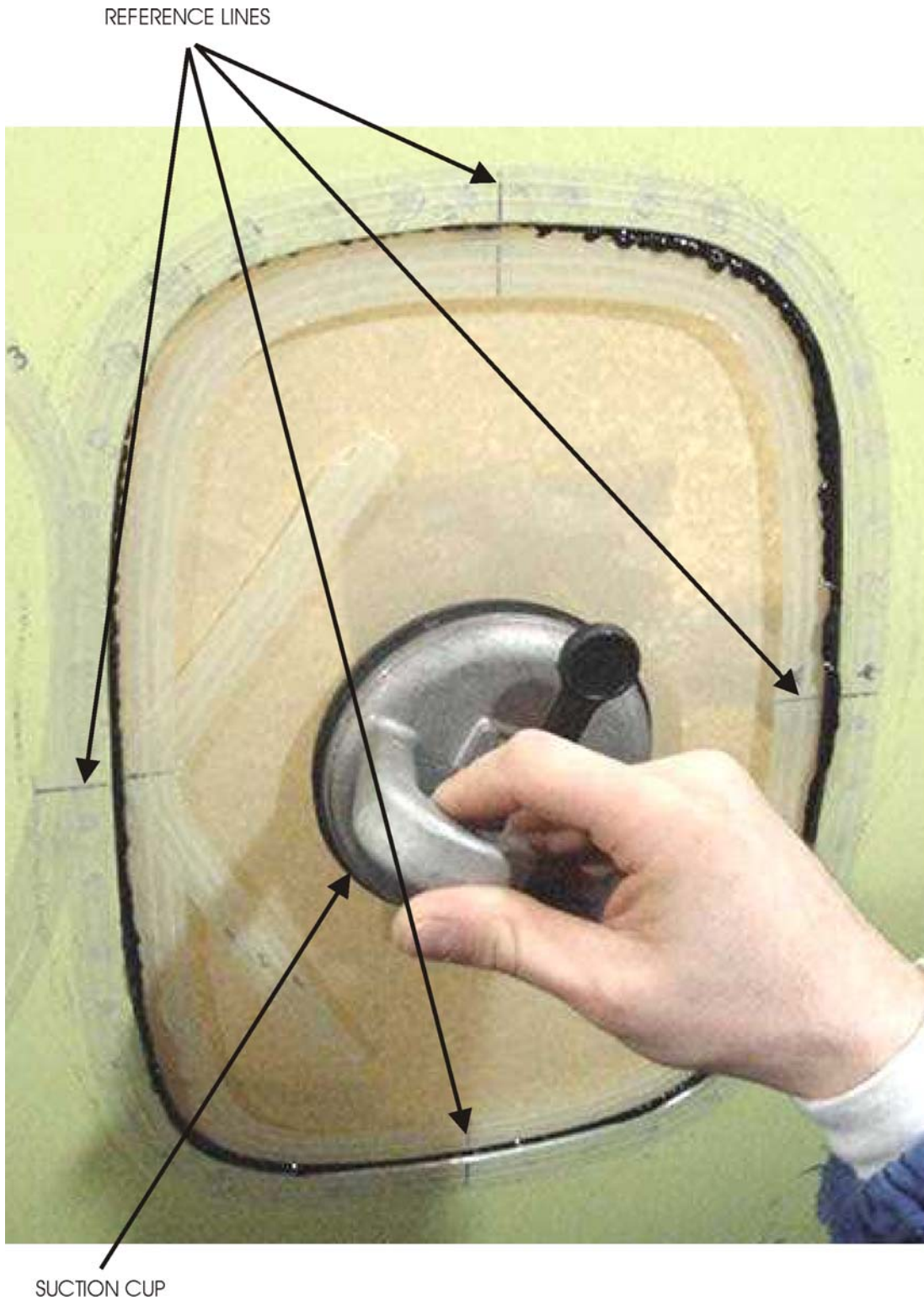
Fig. 201 - Cabin Window - Installation (Sheet 7 of 10)
