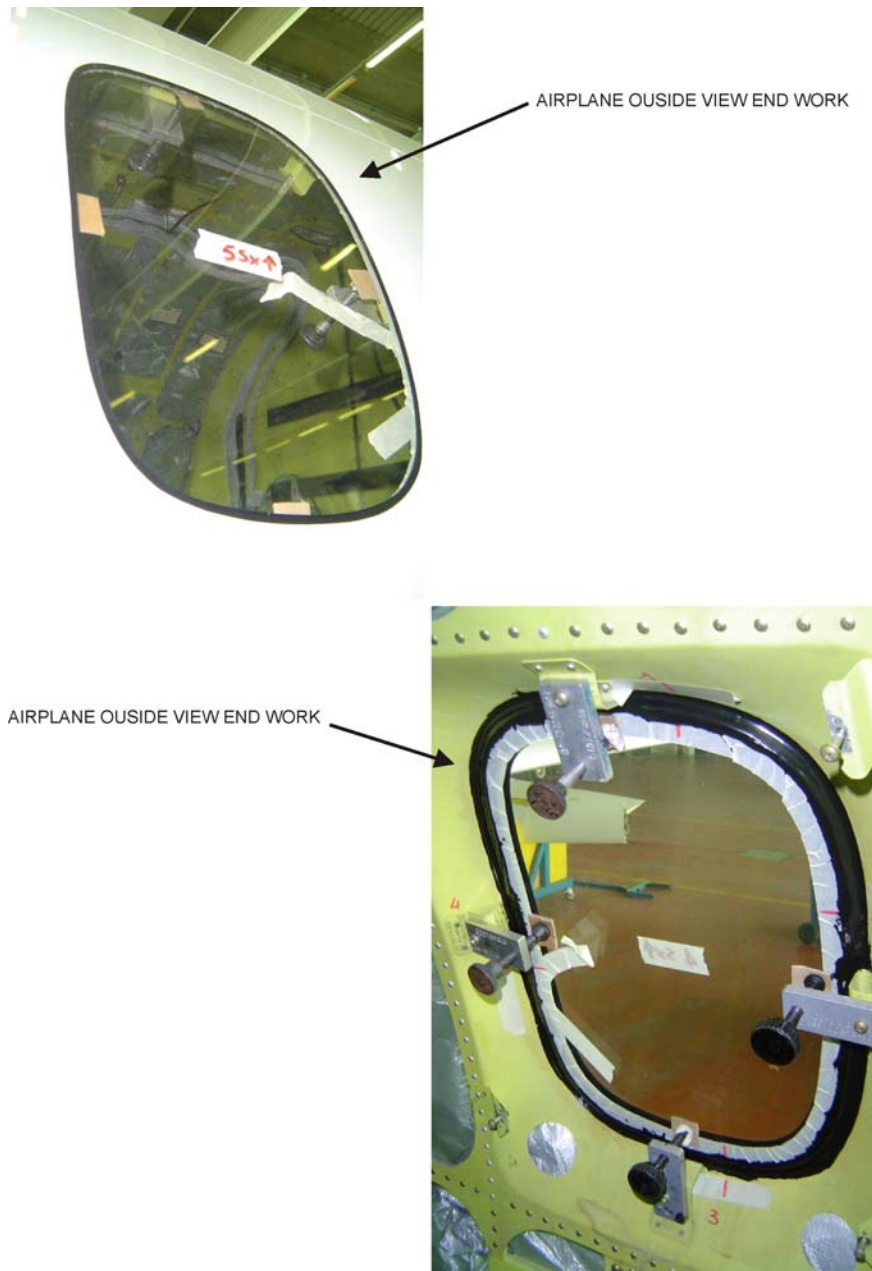
Fig. 201 - Cabin Window - Installation (Sheet 9 of 10)
