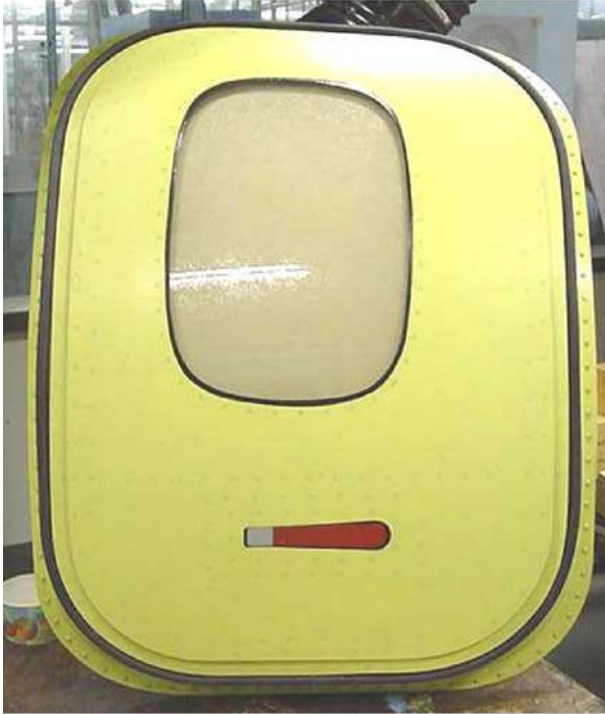
EMERGENCY EXIT DOOR WINDOW EXTERNAL VIEW
