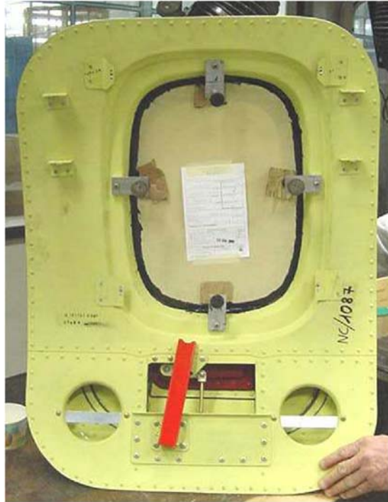
EMERGENCY EXIT DOOR WINDOW INTERNAL VIEW
