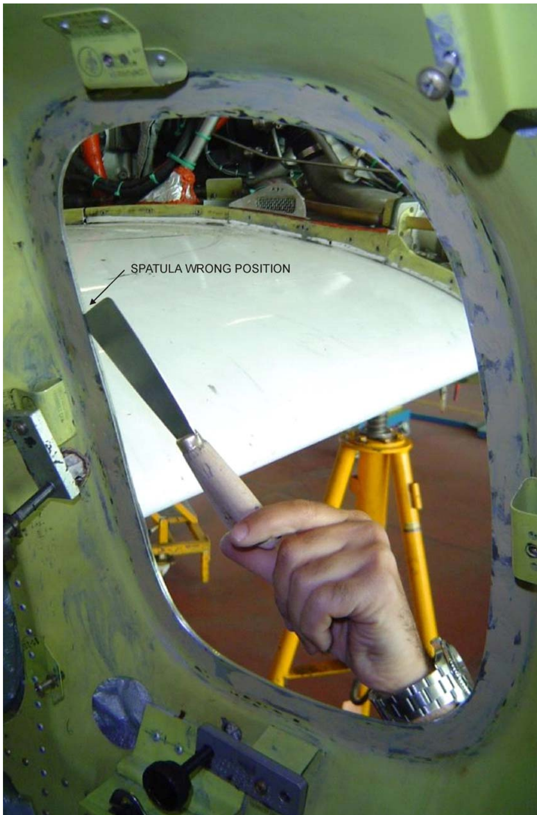
Fig. 201 - Cabin Window - Removal (Sheet 2 of 10)
