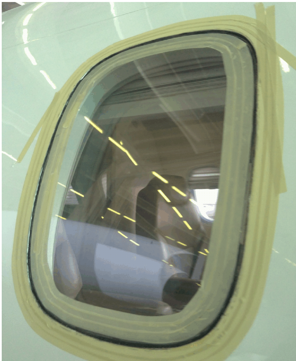
Fig. 205 - Cabin Window External Sealant - Restore (Sheet 3 of 4)
