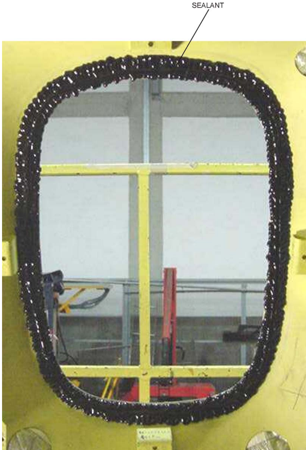
Fig. 201 - Cabin Window - Installation (Sheet 6 of 10)
